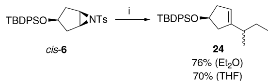
Scheme 7. Reagents and conditions: (i) 2.9 equiv. s BuLi, Et 2 O or THF, –78°C, 4 h then to rt over 1 h.
